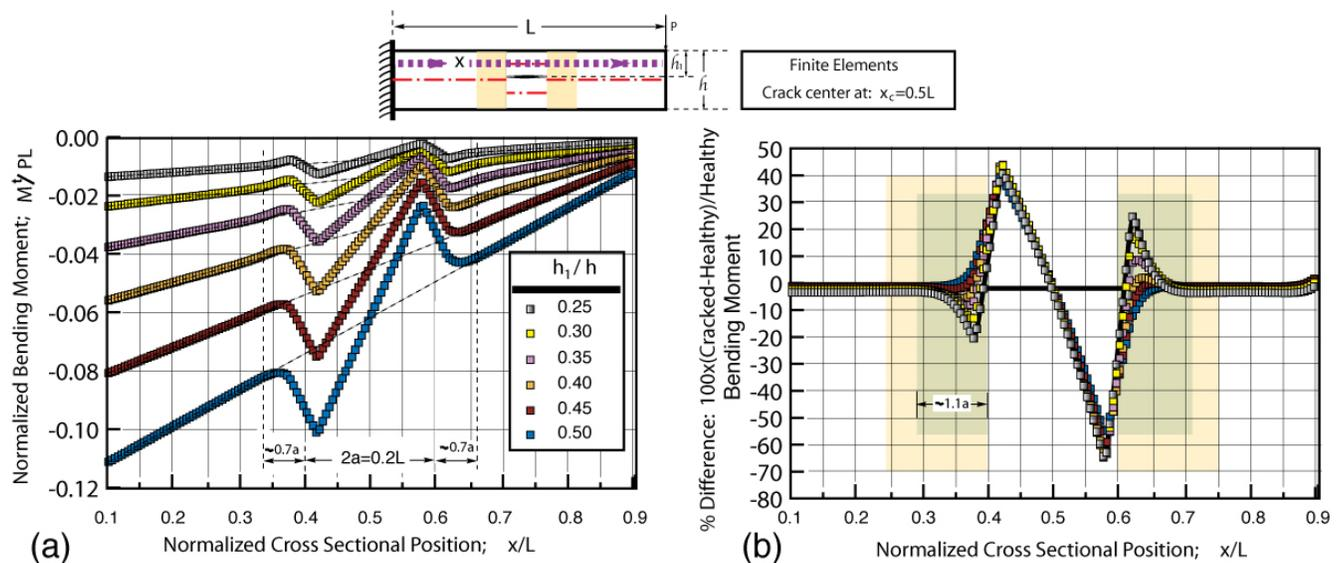
**Fig. 9.** (a) Profiles of the normalized bending moment carried by the “top” portion of the beam extracted from the FE models discussed in this study. Different curves correspond to beams with cracks placed at different  $h_1/h$  depths as indicated in the figure. (b) Profiles of the % difference of the bending moment carried by the top portion of the cracked beam to its “healthy” counterpart.
