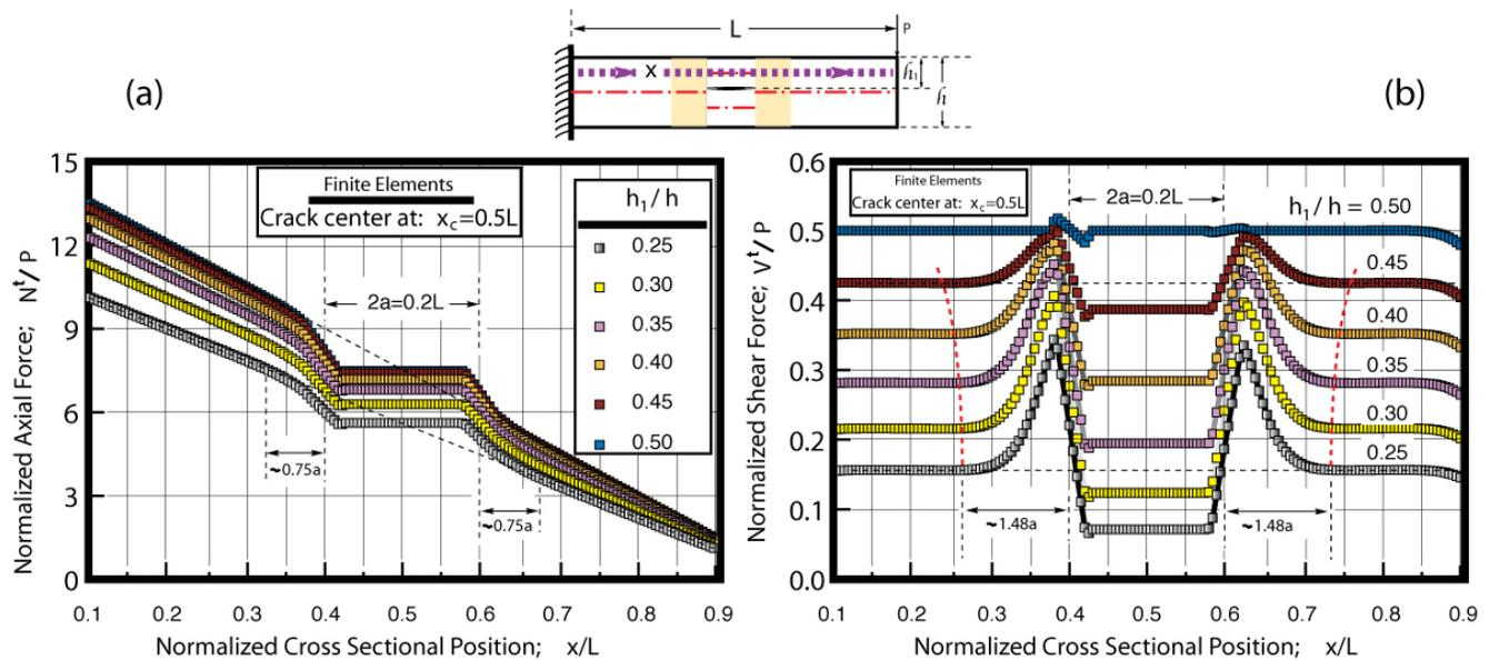
**Fig. 10.** Finite element profiles of the normalized axial force (a) and shear force (b), transmitted through the top portion (i.e., beam above the crack plane) of the cracked beam. The different curves correspond to beam systems containing a horizontal crack at different depths  $h_1/h$  as indicated in the figure.
