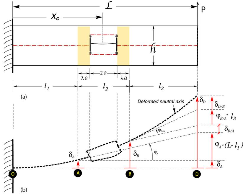
**Fig. 3.** A schematics showing (a) the original cracked beam with its un-deformed neutral axis and (b) the deformed neutral axis configuration of the four-beam model. The relationship between the deflections and rotations at key reference points of the beam are also shown in (b). The deformations and rotations between A and B include the transition zone affects captured by the rotary spring and Timoshenko shear effects.
