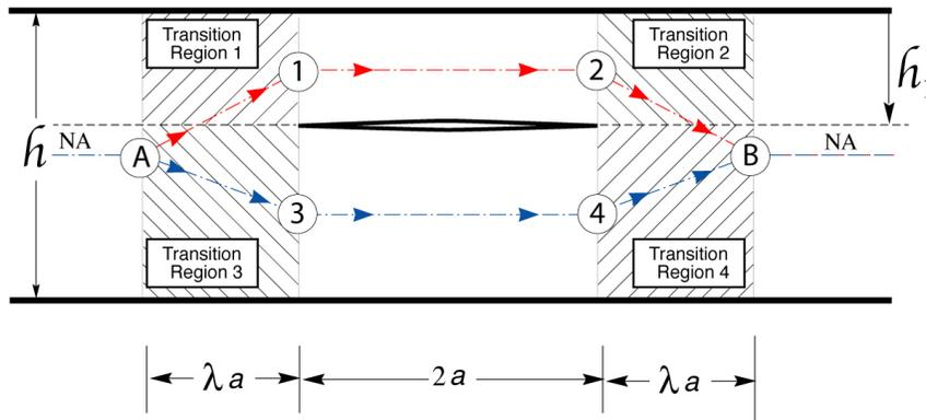
**Fig. 2.** The compatibility paths followed through the “top” and “bottom” beams in establishing angle of rotation and deflection compatibility conditions from reference section A to reference section B. Also shown are Transition Regions 1-4.
