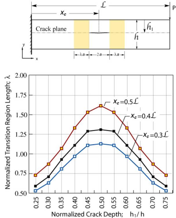
**Fig. 8.** The non-dimensional transition region length parameter  $\lambda$  plotted against the normalized crack depth  $h_1/h$ . Results obtained through the four-beam model for three different crack locations, i.e.,  $x_c/L = 0.3, 0.4$  and  $0.5$  are presented. The discrete symbols represent the cases for which finite element deflections at the free end of the beam were used to solve for the crack length parameter  $\lambda$ .
